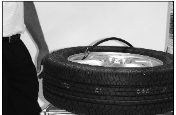
Figure 20 - Stand Back during Bead Seat
