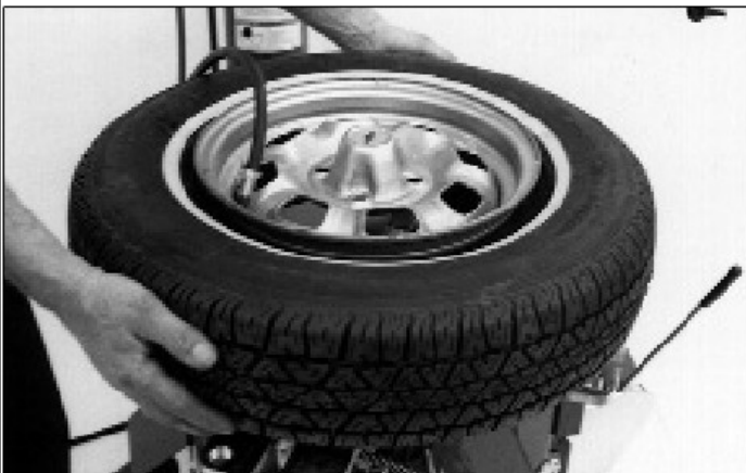
Figure 19 - Lift Tire Upwards for Bead Sealing
