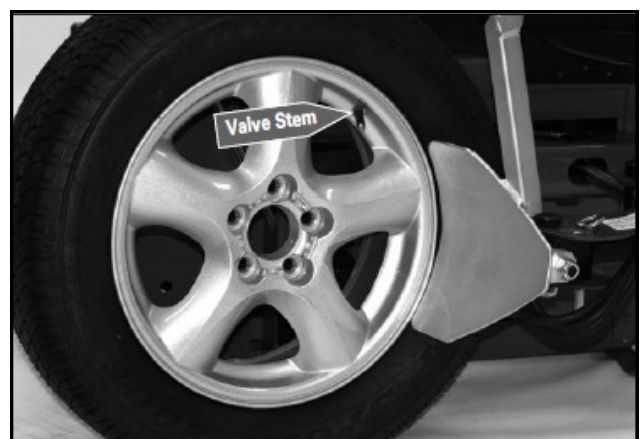
Figure 3 - Position Tire and Bead Loosener Shoe
